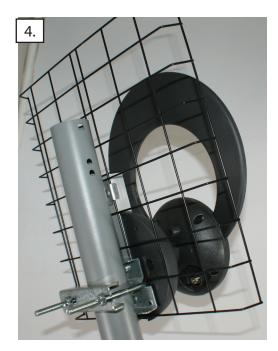
**4. Assembly complete.** Attach the C1 antenna to any kind of mast or mount (up to 2" in diameter) with the adjustable U bolt clamp. The 75 ohm coax connector is in the center rear.
